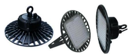
APPLICATION Watertight luminaire, for storage yards, working spaces, industrial areas etc TECHNICAL DATA Protection degree: IP 65/66 Color Temperature:3000K-3500K-4000K-4500K-6000K-6500K. Power factor: ≥0,90 Shine Angle:90°C Driver: CE Waterproof LED Chips: Bridgelux 2835/3030 140pcs SMD 1W Voltage: AC 85V-305V Surge Protector: 4000V CE Certificate Warranty: 5 Years
