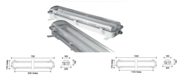
Body: Zinc coated Steel Paint: H Anti-UV, Paint Powder coating with high resistance at the corrosion Cover: Polycarbonate Ingress Protection: IP66 Clips: INOX Lamps Holder: G13 Lamps Type: T8 LED TUBE
